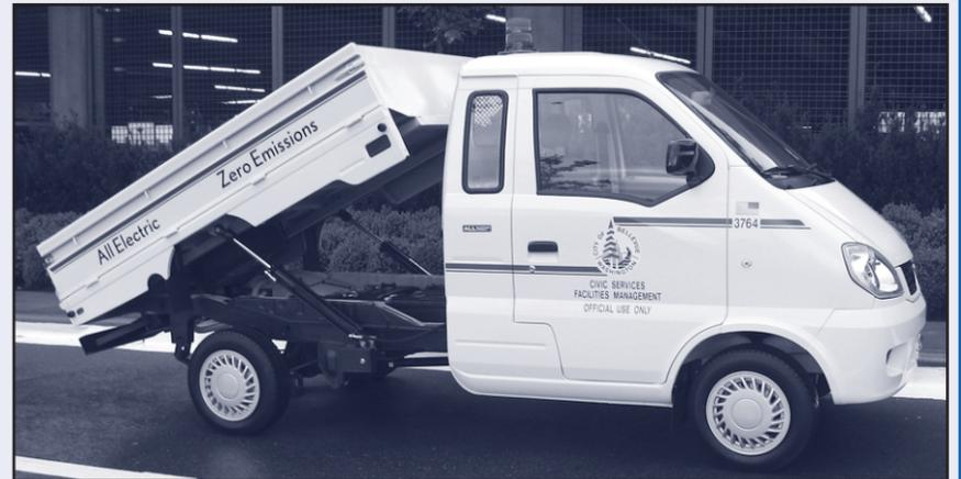
Made by Miles Electric Vehicles of Santa Monica, Calif., the truck has six large batteries and plugs into a regular outlet. Charged overnight, it is ready to roll in the morning.
