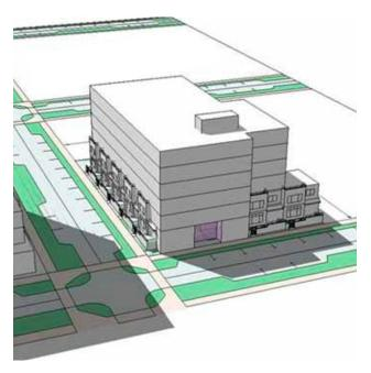
Figure 3.6 The illustration shows a prototypical six story (5 over 1\*) infill building with 80 residential units.
