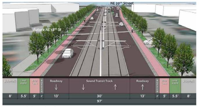
Figure 5.11 136th Place NE planned cross section
