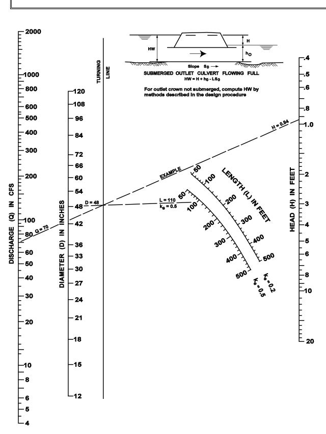
Figure 4.12 Head For Culverts (Pipe W/''*N*''= 0.012) Flowing Full With Outlet Control
