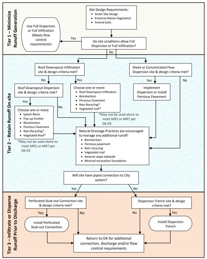
Figure 6.1. On-site Stormwater Management Facility Selection for MR5 and MR7.
