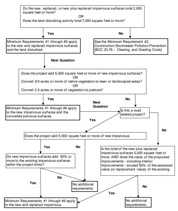
Figure 2.3 Flow Chart for Determining Requirements for Redevelopment
