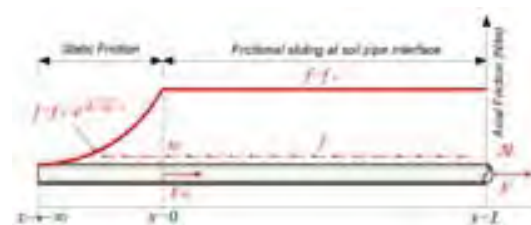
Figure 5. Schematic representation of the axial forces and elongations acting in the pipeline segment away from the fault.
