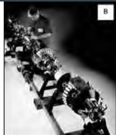
Figure 5: Transverse MFL tool: A) Schematic of the magnetization arrangement for transverse-field, and B) Transverse field tool capable of detecting cracks (Courtesy for TranScan).
